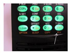
To activate the function, press and hold the **[CLEAR]** key for two seconds.
