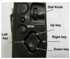
6. Rotate the dial knob or use the RIGHT / LEFT ARROW key to select the desired CTCSS tone from the range of 67.0 Hz ~ 254.1 Hz as shown on the chart. The current CTCSS tone is displayed on the LCD.
