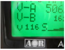
7. "v nnn" will appear on the bottom left of the LCD while the VOICE INVERTER function is activated.
