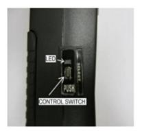
4. To stop recording, press and hold the [CONTROL] switch again for two seconds. The red LED will go off.
