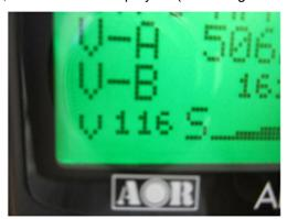
5. Rotate the squelch knob counter clockwise to display "S" icon on the centre bottom of the LCD. The background squelch noise will be heard.
