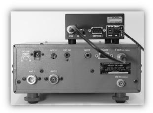
Each unit needs its own power source; therefore you will need to supply the power source for ARD300. If you happen to own the AR8600MK2 receiver, you can use its AC adapter AA8600. (The AA2300 adapter of AR2300/5001D/6000 can be used as well)
