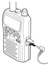
5 Insert the AC adapter power plug into an AC outlet (100 V-240 V).
