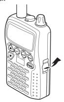
Insert the DC output plug into the external DC jack on the right side of the AR-mini.
