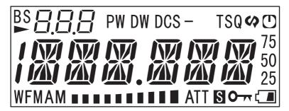
1: This segment appears when the frequency in VFO is 1000 MHz or higher.
