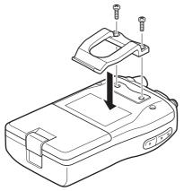
**2** Fix the belt clip with the supplied screws.
